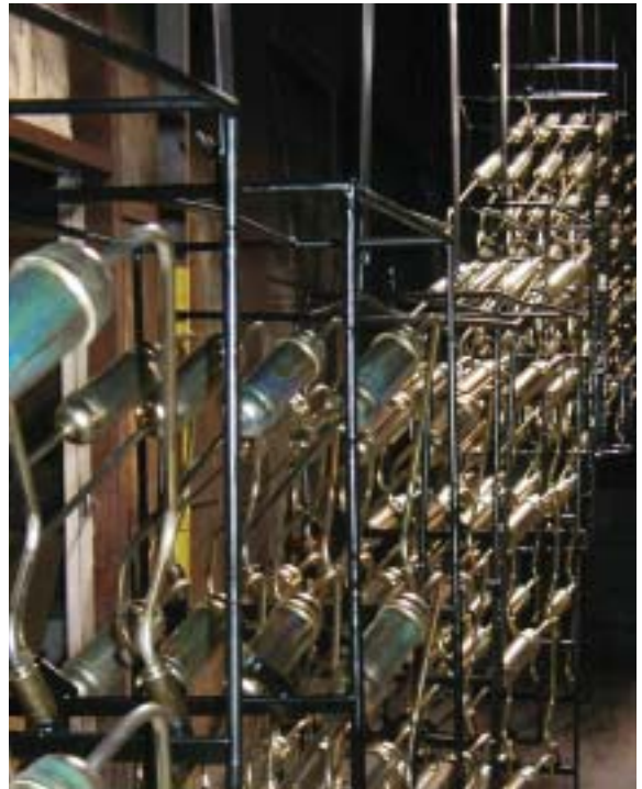
These raw parts have been loaded and are approaching the five-stage washer.
