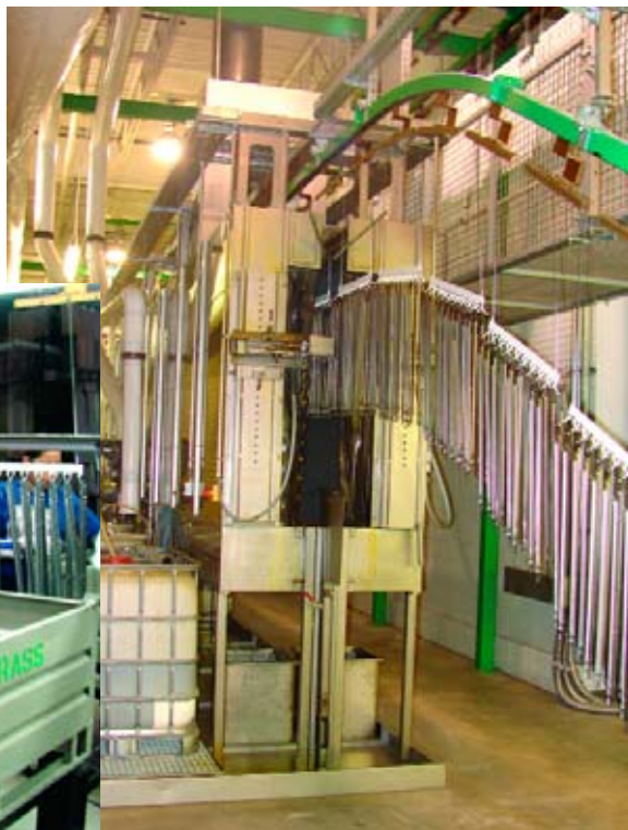
After workers load the drawer slides onto racks, the line takes the parts through a four-stage washer.
