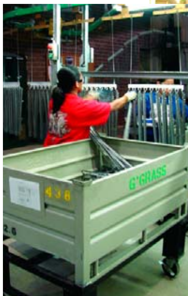
After workers load the drawer slides onto racks, the line takes the parts through a four-stage washer.
