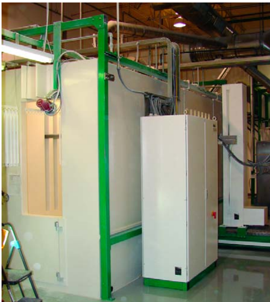
Automatic guns on reciprocators powder coat these drawer slides.
